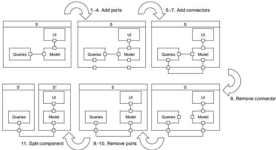
Figure 6: Complex refactoring on architectural level
