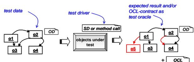
**Fig. 2.** Structure of a test modeled with object diagrams (OD), sequence diagram (SD) and the Object Constraint Language (OCL).
