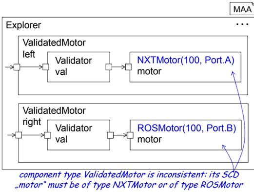
Fig. 4. Example for a clash between the two bindings  $\text{left.motor} \rightarrow \text{NXTMotor}(10, \text{Port.A})$  and  $\text{right.motor} \rightarrow \text{ROSMotor}(10, \text{Port.B})$ , which our transformation resolves.
