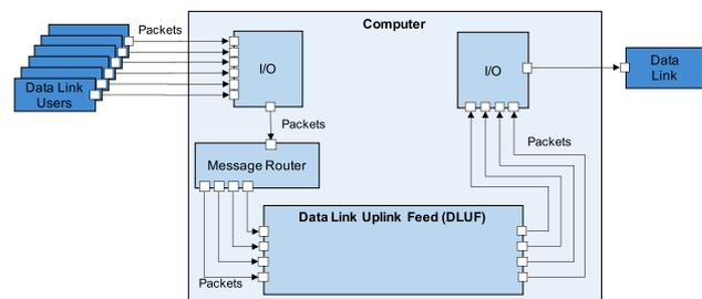
**Fig. 2** Graphical representation of the DLUF system context[57]
