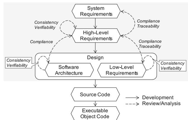
**Fig. 1** The MontiBelle approach provides means to guarantee the **a** compliance, **b** consistency, **c** verifiability, and **d** traceability between SRs, HLRs, software architecture, and LLRs in the systematic design as suggested by EUROCAE ED-216
