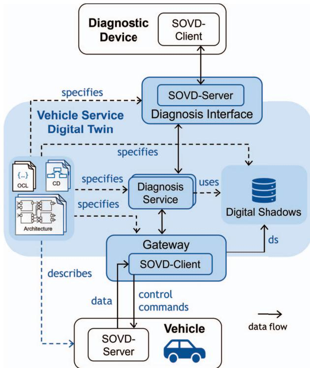
Fig. 5. The DT of a single vehicle service; model-driven engineering is utilized to generate digital twin parts from architecture diagrams, class diagrams, and OCL.
