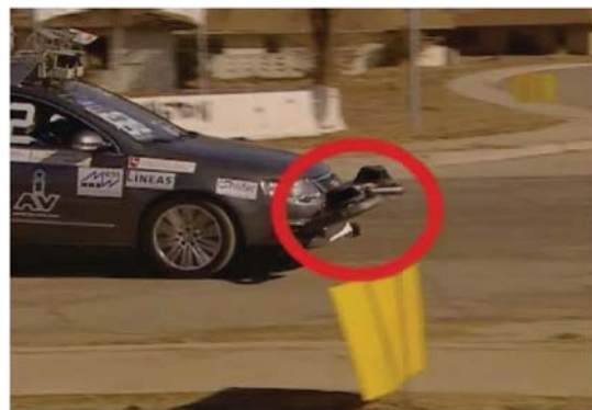
(b) The red circle shows the twisted carrier rod.
