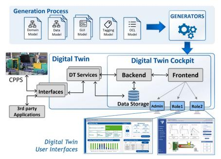
Fig. 3: Artifacts of the MontiGem generator framework to generate a digital twin cockpit with multiple interfaces according to each role of the end user.
