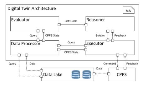
Fig. 2 Reference architecture for self-adaptive digital twins [BDH+20]
