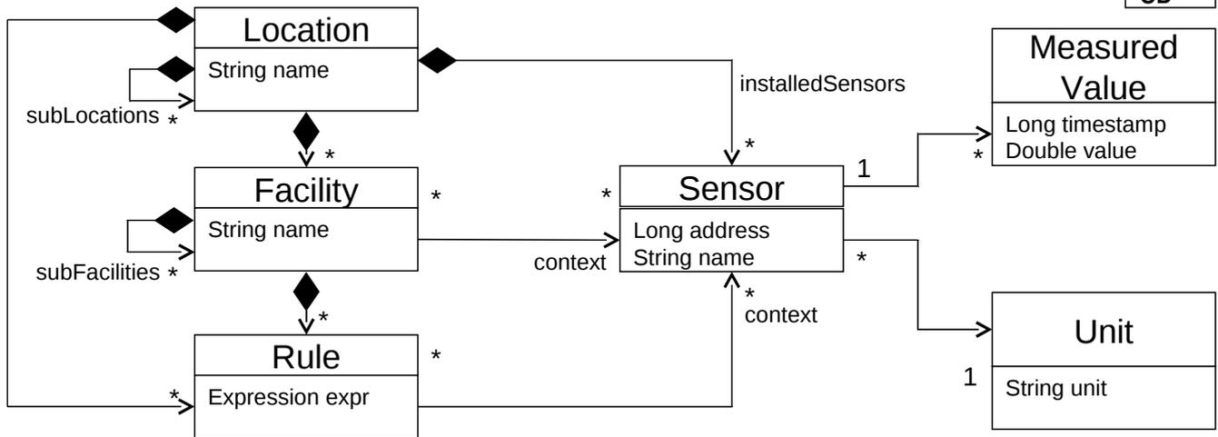
Figure 2: Domain model as class diagram
