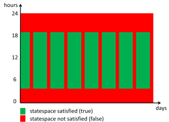
Figure 6: A carpet plot showing at what points of time the state space is satisfied or not satisfied
