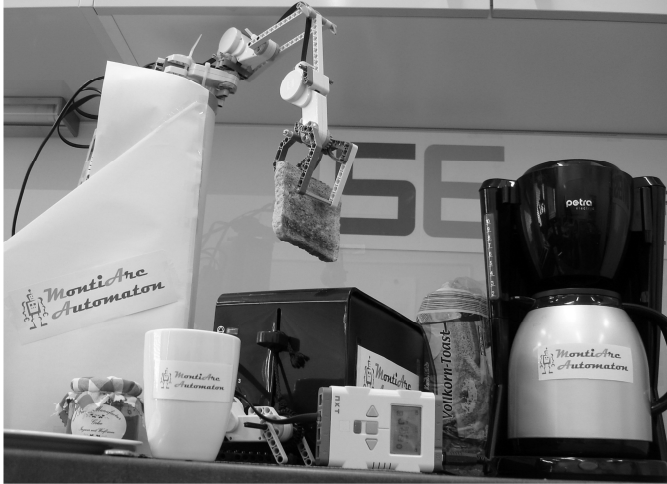
Fig. 2: Lego NXT hardware and environment of the Toast-ServiceRobot application.
