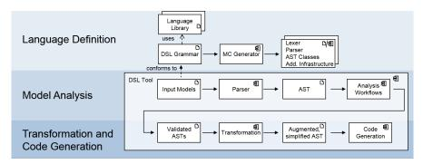
Figure 3 – The role of DSLs in a model-based software engineering process.
