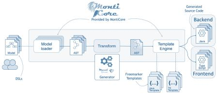
Figure 16 – Overview of the generator components
