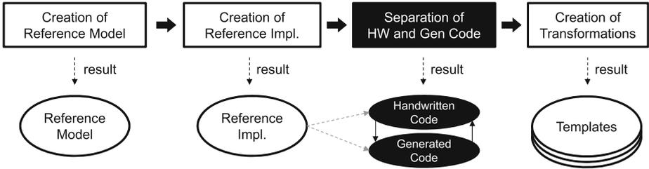
**Fig. 1.** Typical development steps of a code generator.
