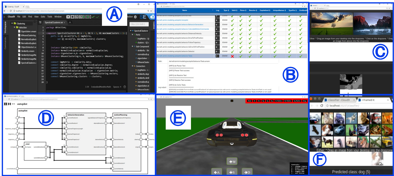
Figure 1: Screenshots of Main Features of EmbeddedMontiArc: (A) IDE, (B) Quality Reports incl. Results of Unit Tests, (C) Image Clustering, (D) Generated Graphical C&C Layout of Textual EMA Models, (E) 3d-Car Simulator Executing Autopilot Controller, (F) Image Classifier based on CNN Models
