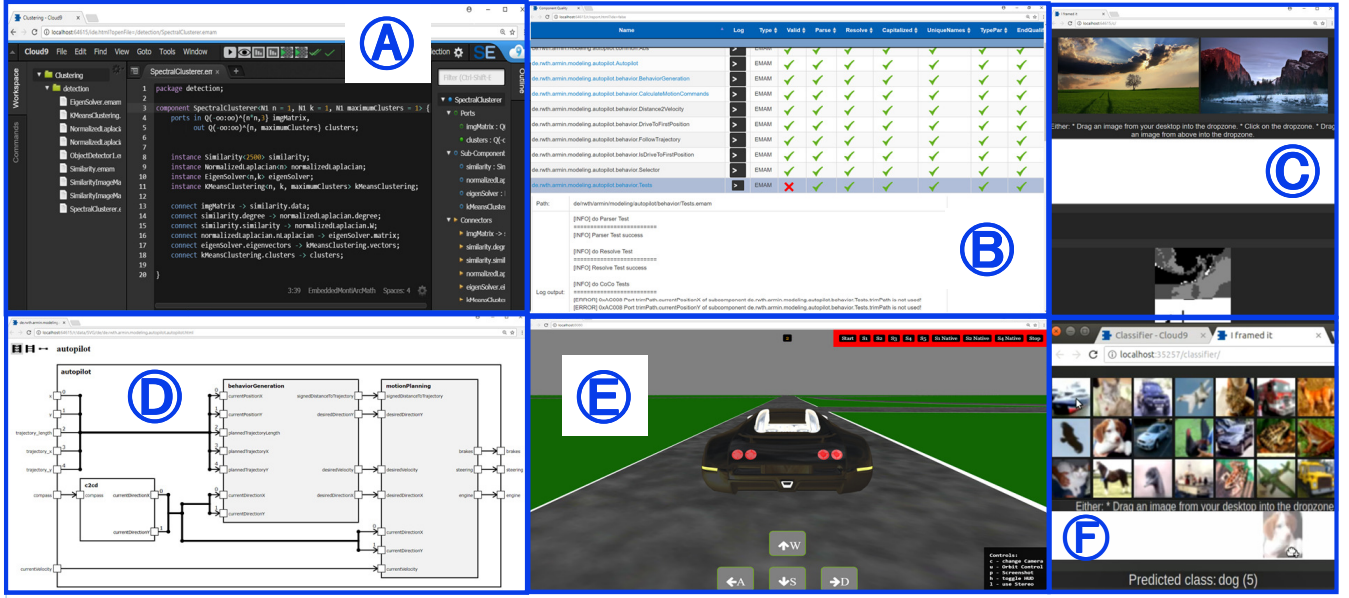
Figure 1: Screenshots of Main Features of EmbeddedMontiArc: ① IDE, ② Quality Reports incl. Results of Unit Tests, ③ Image Clustering, ④ Generated Graphical C&C Layout of Textual EMA Models, ⑤ 3d-Car Simulator Executing Autopilot Controller, ⑥ Image Classifier based on CNN Models
