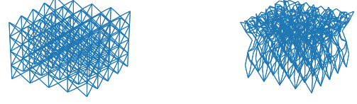
Figure 4: Initial and deformed Lattice structures
