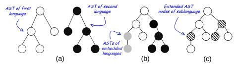
**Fig. 2.** The resulting abstract syntax trees (ASTs) when using (a) aggregation, (b) embedding, and (c) inheritance. Aggregation results in separate ASTs for each model. Embedding results in a single AST with subtrees embedded at the leaves of the host language. Inheritance results also in a single AST containing extended nodes of the sublanguage.
