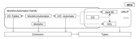
**Fig. 3.** An overview of the MontiArcAutomaton integration. Rounded corners show language aggregation. All other boxes show languages. Dashed arrows mark language embedding. Solid arrows mark language inheritance. The CD language is part of both the UML/P and the MontiArcAutomaton family aggregation.
