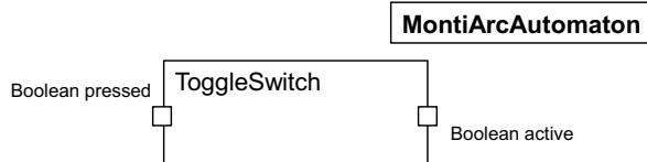
Figure 6.11.: The component ToggleSwitch with input port pressed of type Boolean and output port active of type Boolean.
